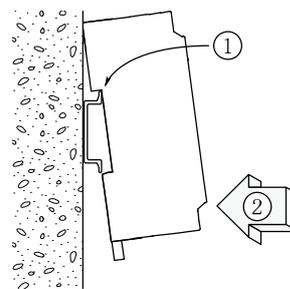
Hold the unit with the slide clamp facing down. Hook the upper edge of the cavity in the rear of the unit over the upper blade of the rail (1), then push the lower part of the unit against the lower blade of the rail so as to make the slide clamp engaged firmly with the rail (2).
