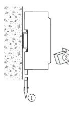
Push the slide clamp downward with a flat-head screwdriver bit or the like (①), and pull the lower part of the unit toward you (②).
