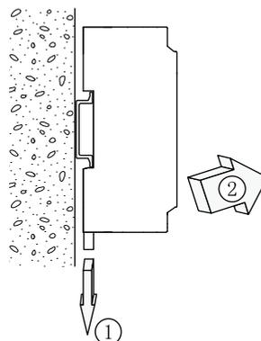
Push the slide clamp downward with a flat-head screwdriver bit or the like (1), and pull the lower part of the unit toward you (2).
