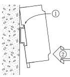
Hold the unit with the slide clamp facing down. Hook the upper edge of the cavity in the rear of the unit over the upper blade of the rail (1), then push the lower part of the unit against the lower blade of the rail so as to make the slide clamp engaged firmly with the rail (2).
