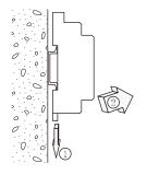
Push the slide clamp downward with a flat-head screwdriver bit or the like (①), and pull the lower part of the socket toward you (②).
