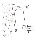
Hold the socket with the slide clamp facing down. Hook the upper edge of the cavity in the rear of the socket over the upper blade of the rail  $(\begin{cal}0\end{cal})$ , then push the lower part of the socket against the lower blade of the rail so as to make the slide clamp engaged firmly with the rail  $(\begin{cal}2\end{cal})$ .
