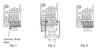
Note: For your safety, do not make any electrical connections or disconnections with power supplied to the instrument. Make sure that all terminal screws are properly tightened each time you finish the tightening.
