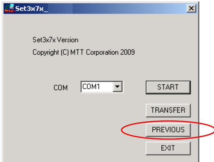
To make configuration to more than one unit of conditioners by [Transfer the previous configuration] button.
