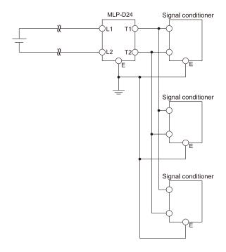
NOTE: If the distance from the MLP device to the equipment to be protected is over 10 meters, it is recommended that an additional MLP device adjacent to the equipment to be protected should be installed.
