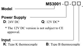
**E**: Type E thermocouple **J**: Type J thermocouple **T**: Type T thermocouple
