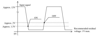
Input code M: Open collector input; threshold voltage: approx. 5V
