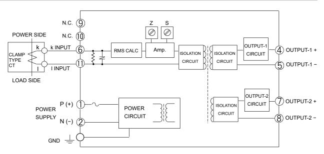
\* The output terminals of the supplied clamp type CT should be connected to the input terminals on the transmitter's terminal block.
