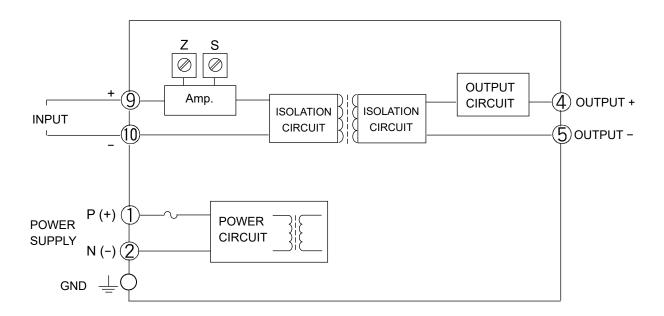
Note: A short circuit between the output terminals (#4 and #5) must be avoided as it may cause a failure.
