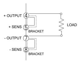
If the wiring resistance for output is too high to be acceptable, the terminal connections should be made without the supplied brackets as illustrated below.
