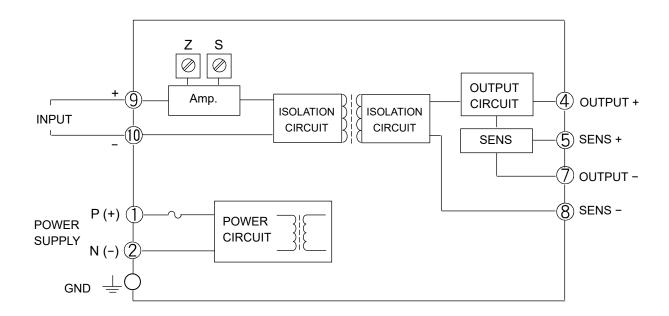
Normally, the terminals + OUTPUT and + SENS (#4 and #5) should be short connected with the supplied bracket. Also, the terminals - OUTPUT and - SENS (#7 and #8) should be short connected with the supplied bracket.
