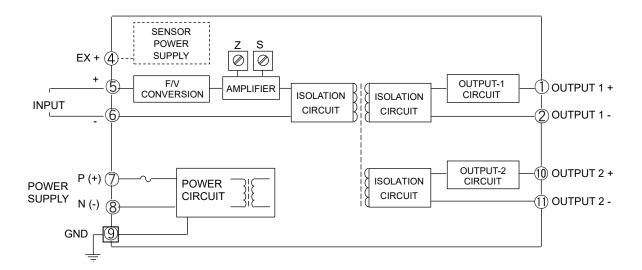
For dry contact or open collector input:
