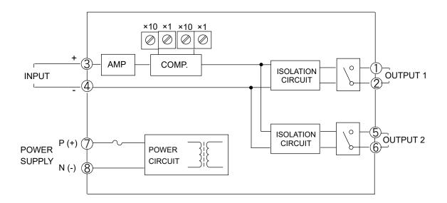
When an inductive load, such as an electric motor, is connected to the output, a relay contact protection circuit must be connected across the load.
