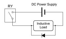
Protection Circuit (Diode, Varistor, CR circuit, etc.)
