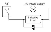
Protection Circuit (Varistor, CR circuit, etc.)
