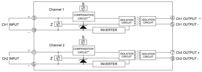
\* CIRCUIT FOR COMPENSATING FOR OUTPUT VARIATION DUE TO LOAD CHANGE
