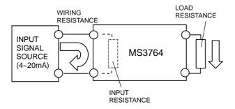
Note: The input resistance for the voltage output model is fixed to approx.  $250\Omega$  (for 20mA DC input).
